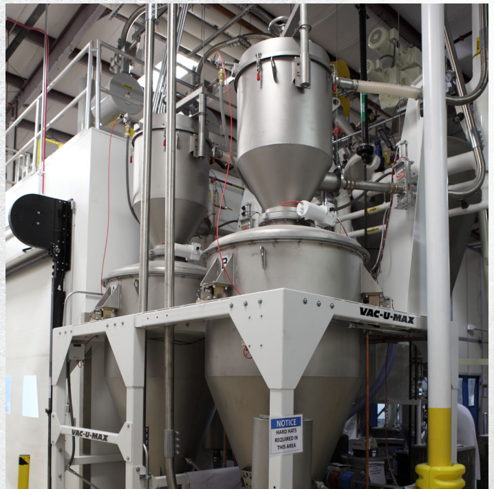
Whether transferring as little as a few pounds per hour or up to 25,000 lbs/hr (11,340 kg/hr), vacuum conveyor performance is determined by the material's flow characteristics and the conveyor's design, ensuring reliable handling across a wide range of powders and bulk solids.
