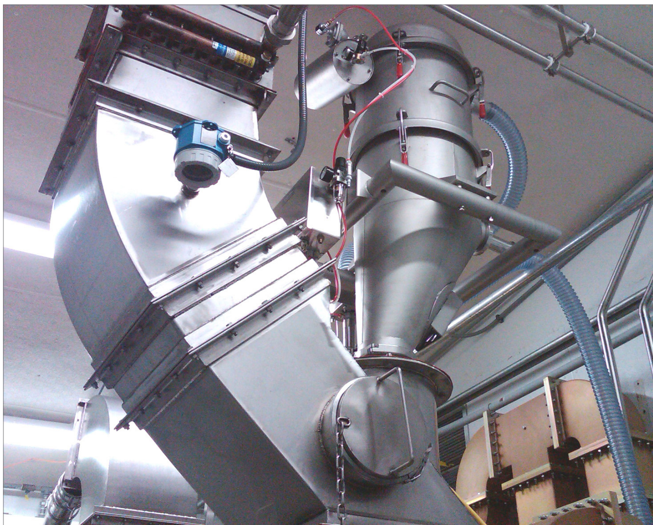
Vacuum conveyor shown as part of a two-stage system: One unit fluidizes and transfers powder to the mixer, while a second unit conveys finished material from the mixer to the next process.
