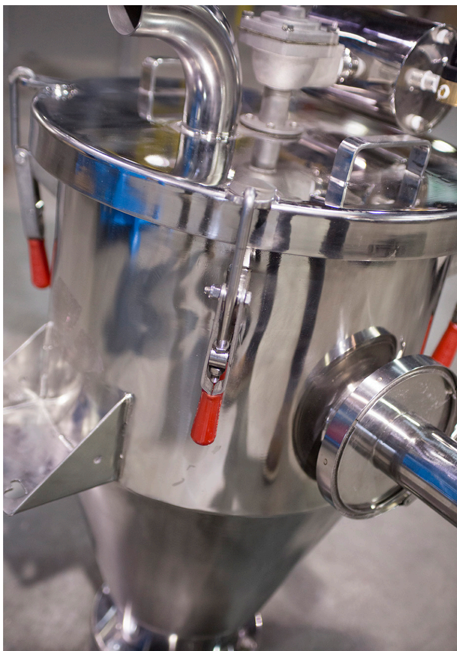
Stainless steel concentric-cone vacuum conveyor, designed for free-flowing powders such as sugar, salt, flour, resins, and other low-cohesion materials.
