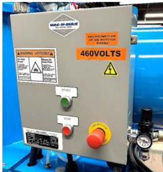
UL -certified 508A control panel with 24VDC pushbuttons for safety
