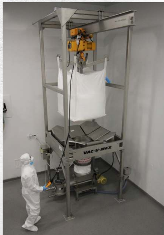
Bulk Bag Unloaders also known as Bulk Bag Discharge Systems, provide an easy, clean, and controlled way to discharge the entire contents of bulk bags.
