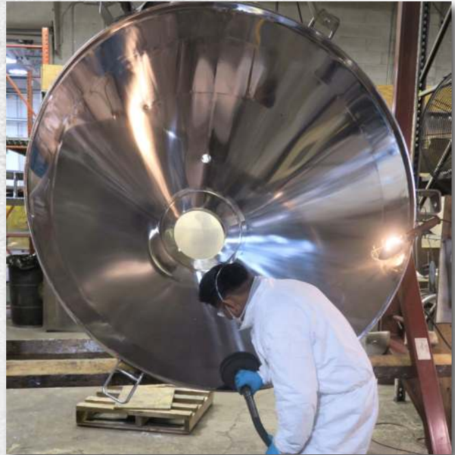
RA25 or lower finish and passivation are standard in the manufacture of sanitary components. rated for NEMA 4X.
