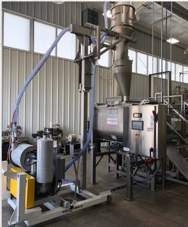
VAC-U-MAX Receiver conveys product to mixer, increasing productivity while greatly reducing sanitizing downtime.
