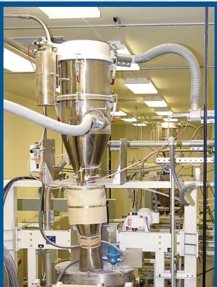
Pharmaceutical Packaging Application Utilizing VAC-U-MAX Receiver
