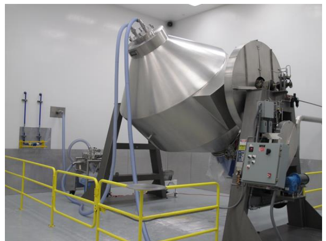
VAC-U-MAX Blender Loading System at a Nutraceutical Company. Conveying Powder to a 150 cubic foot GEMCO Blender.
