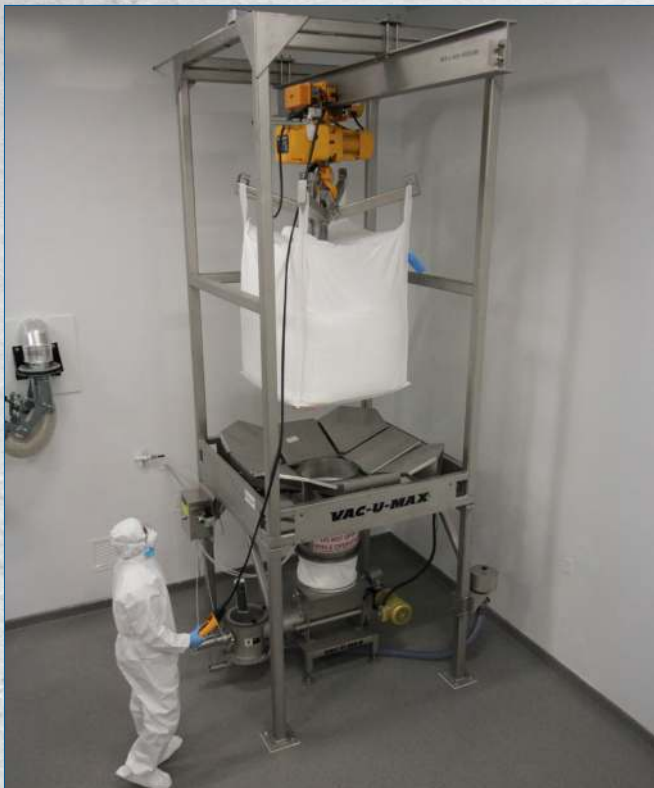
VAC-U-MAX Activator™ Bulk Bag Unloading System features four "No Maintenance" actuator petals that massage the lower portion of the bag alternating side-to-side pattern promoting optimal material flow to center of bulk bag.
