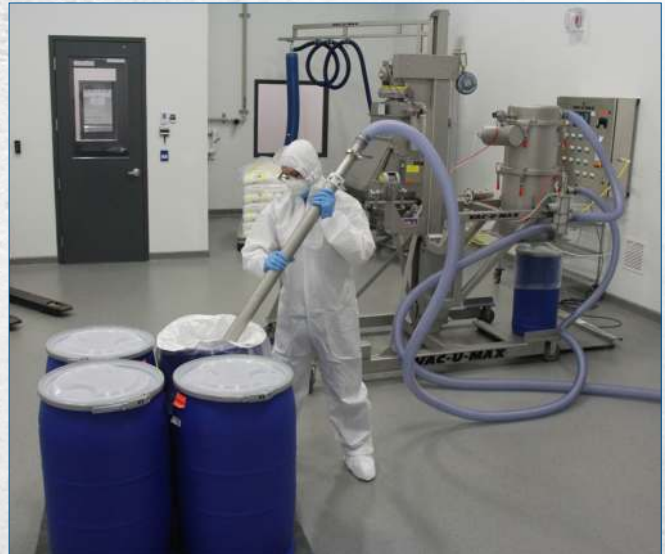
Operator transfers ingredients from commercial containers with a wand and vacuum conveyor, conveying material into hygienic drums which meet specific weights.
