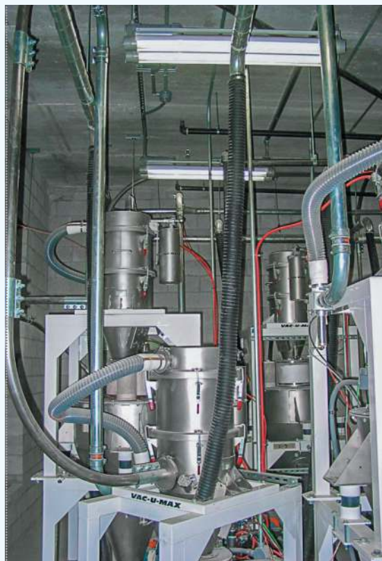
Your conveying process may be batch or continuous. Shown here is a continuous process whereby the vacuum conveying system transfers bulk materials to a weigh hopper on load cells.
