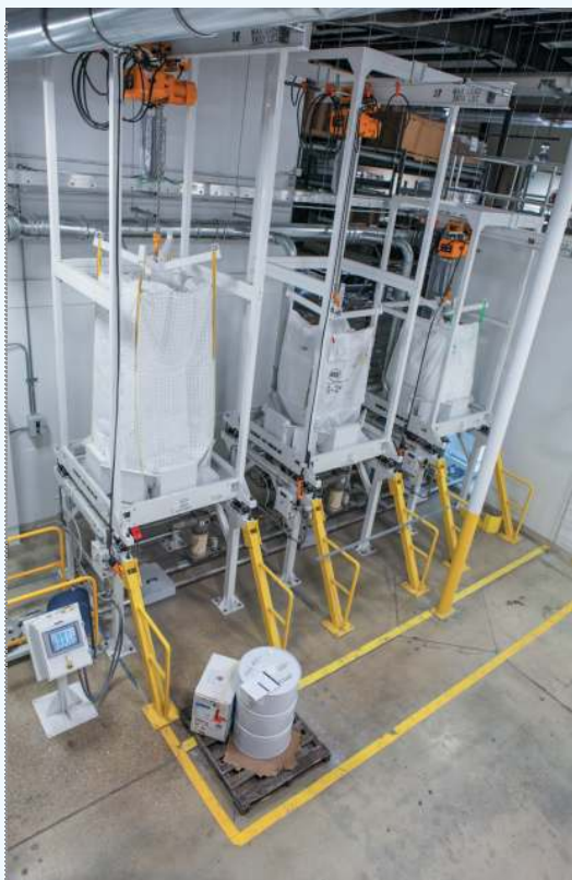
To maximize dust control, bulk-bag unloaders incorporate enclosed vacuum conveying lines, and bag-dump stations integrate dust collectors.
