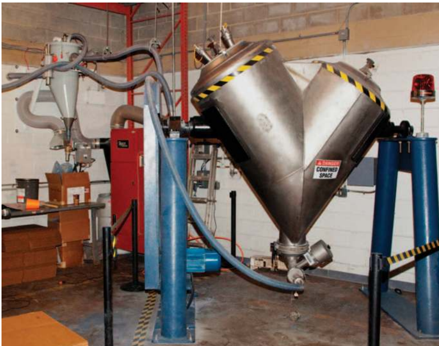
The new direct charge loading system allows the company to load and unload the blender with one system.
