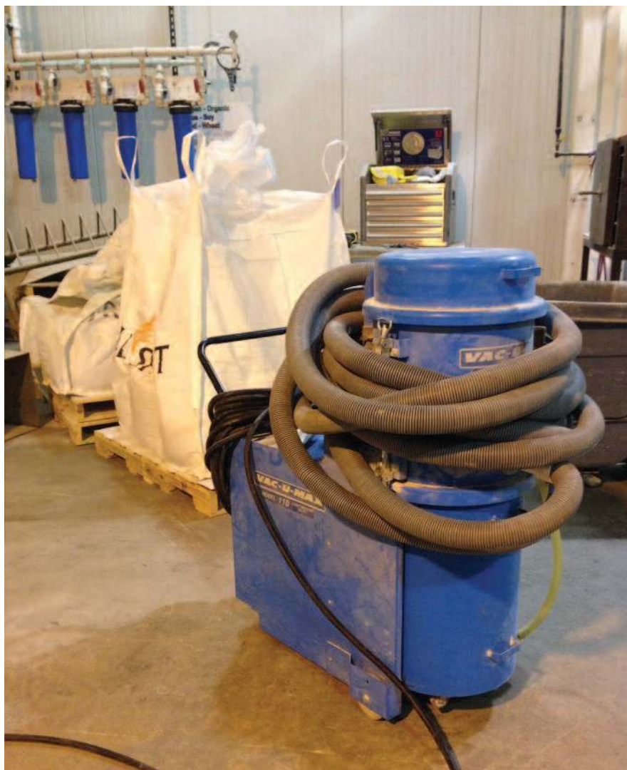
The vacuum can be used by an operator up to 50 feet away from the unit.
