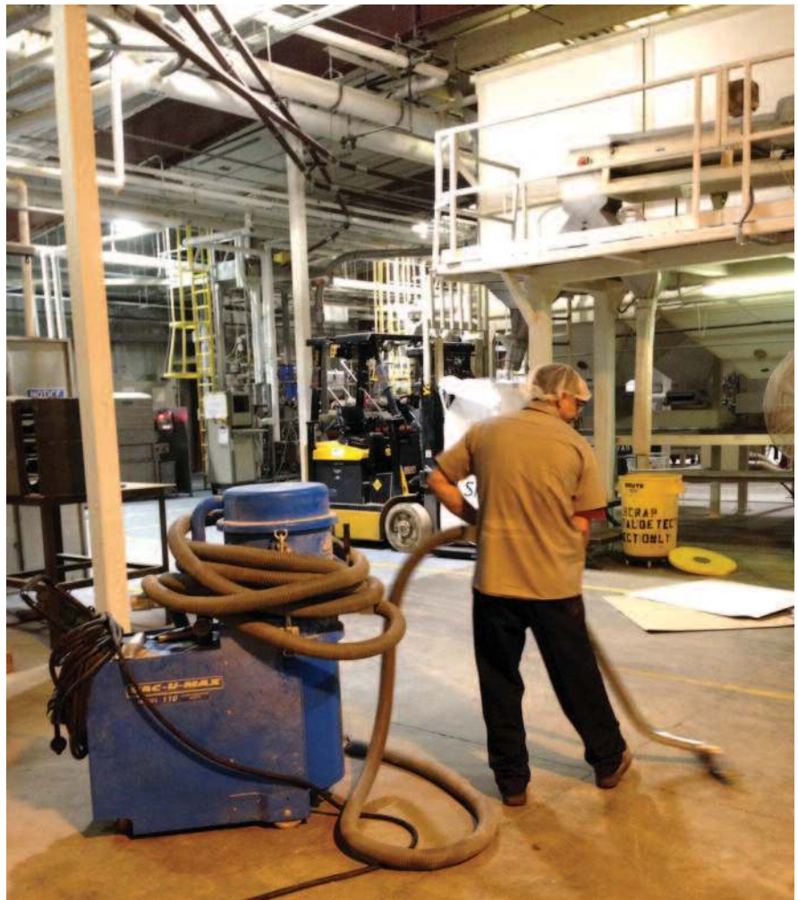
J.R. Short Milling uses portable vacuums for rapid cleanup of fugitive dust from floors, walls, and machine surfaces.
