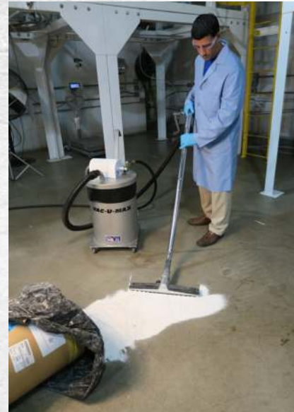
The MDL15 features a 15-gallon collection drum and VAC-U-MAX Venturi power unit which has the lowest compressed-air consumption on the market today.
