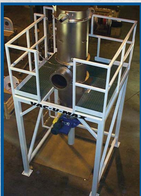
VAC-U-MAX Central Vacuum System with Explosion-Proof Venting
