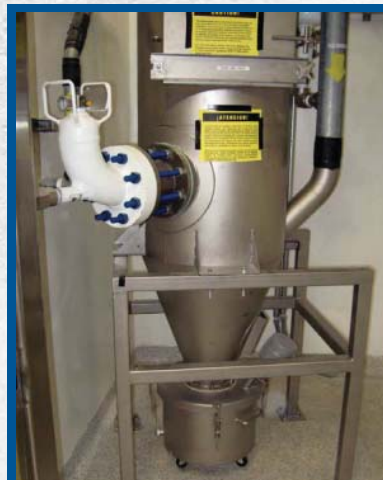
VAC-U-MAX Filter Separator with HRD Chemical Explosion Suppression
