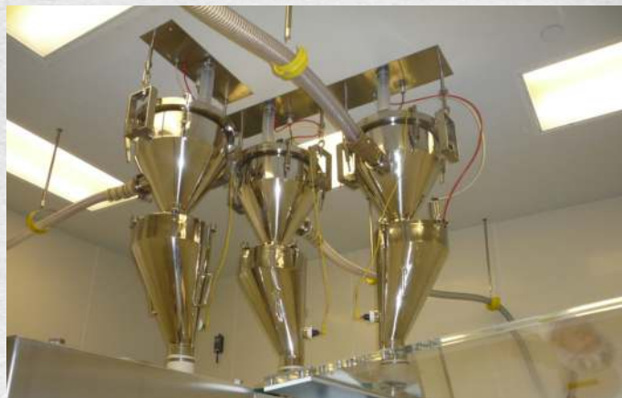
Pneumatic Conveying System with Small Footprint, Eliminating Need for Workers to Climb Steps to Manually Dump Materials into the Process, Making it Safer for Workers
