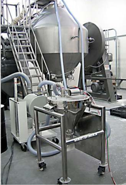
Direct Charge Blender Loading System - a "Better Way" to Move a Variety of Bulk Materials, Eliminating Manual Handling
