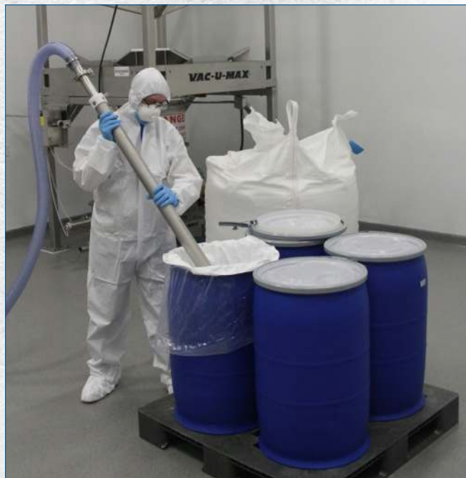
Pickup wand and vacuum conveyor pneumatically convey materials from drums and other sources.
