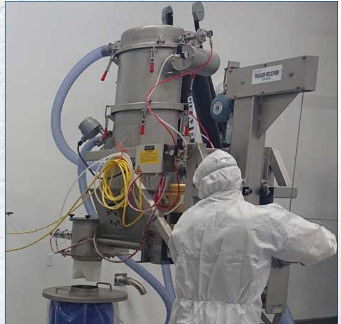
VAC-U-MAX Sanitary Vacuum Conveyor mounted on rolling frame allows mobility and equipment access.
