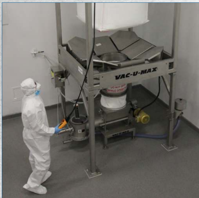
VAC-U-MAX Activator™ Bulk Bag Unloading System features four "No Maintenance" actuator petals that massage the lower portion of the bag alternating side-to-side pattern promoting optimal material flow to center of bulk bag.
