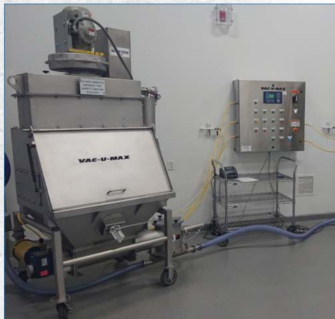
VAC-U-MAX sanitary design Bag Dump Station with integrated dust collection system which automatically turns on when the door is lifted.
