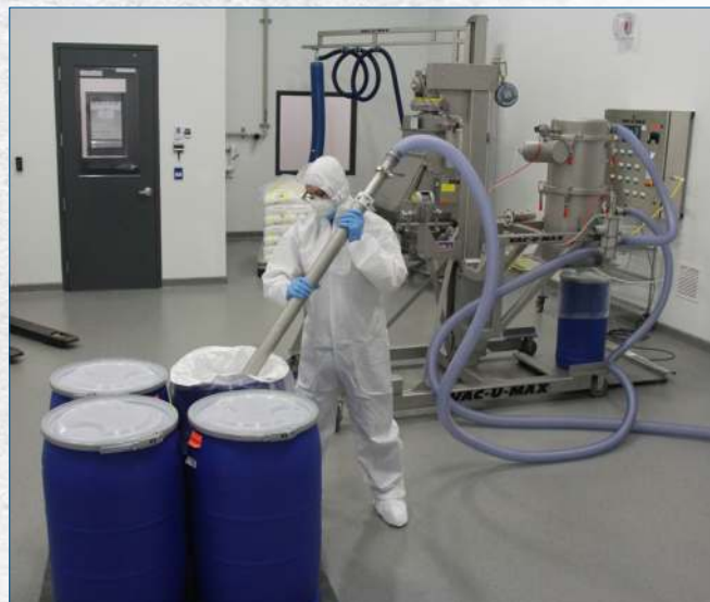
Operator transfers ingredients from commercial containers with a wand and vacuum conveyor, conveying material into hygienic drums which meet specific weights.
