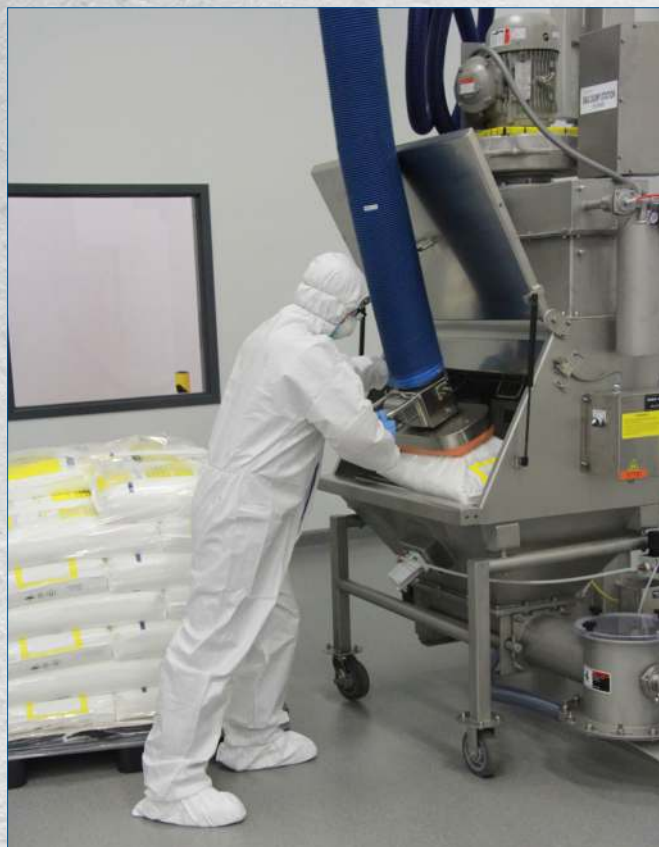
VAC-U-MAX LoadLifter lifts bags from pallet, placing them on a grate inside a VAC-U-MAX Bag Dump Station with integrated dust collection system.
