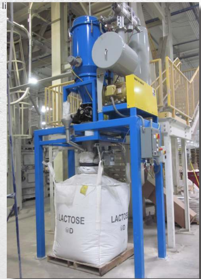
Central vacuum cleaning system with source capture and reclaim into bulk bag for potential reuse, recycle, or disposal.
