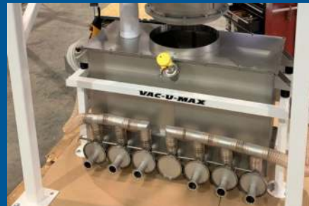
Feedbin with multiple outlets
