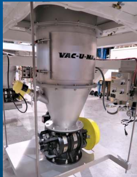
Rotary Valve Discharge on a BBU
