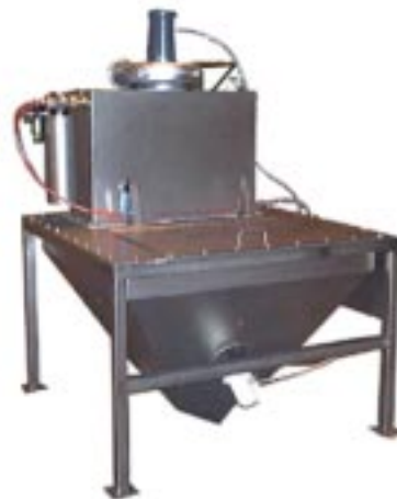
Custom Bag Dump Station with 45degree walls and integral dust collector.
