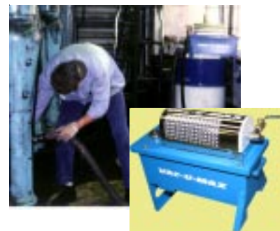
MDL TK, Liquid Only Recovery, 1-2 gallons per second. Fills entire closed top drum
