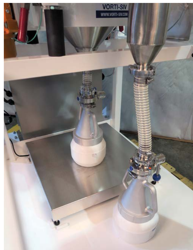
Vac-U-Max on-board sieve and scale separate and weigh reusable powders into industry-standard pail. Oversize/waste debris is also collected (right).
