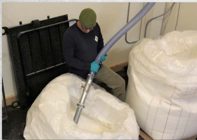
Bulk Bags with vacuum wand replace stair climbing and manual dumping of (30) 50lbs bags, twice per day.
