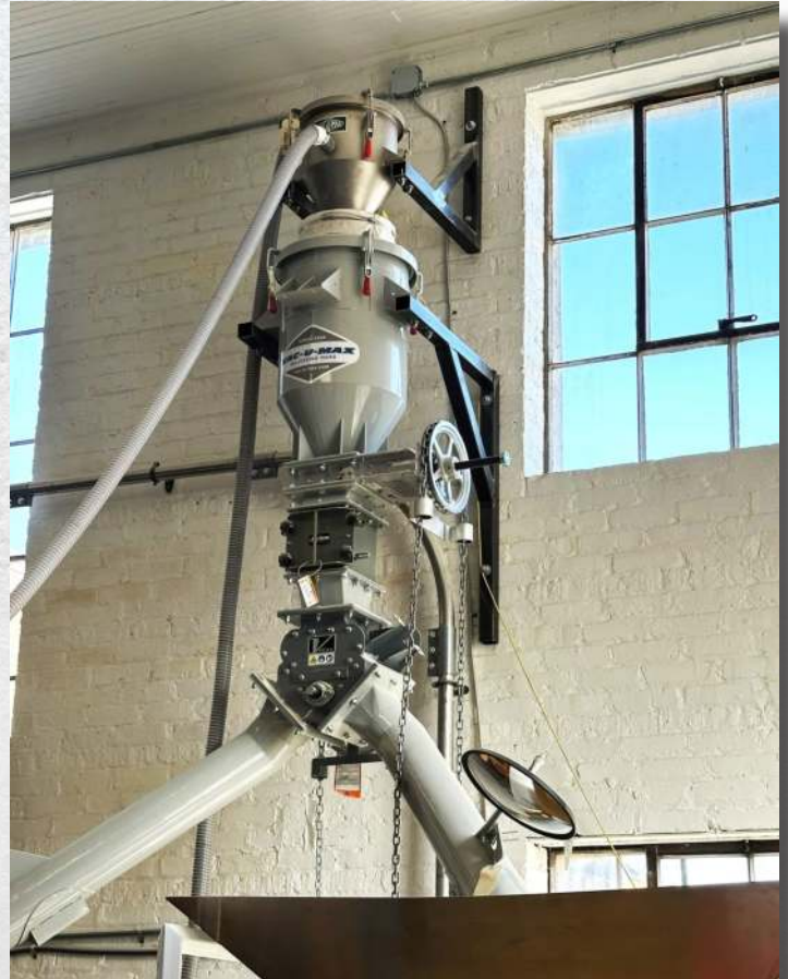
Whole grains from the vacuum receiver are discharged through a magnet and diverter valve to one of the two cold stone mills. Handwheel-operated valves control the flow.
