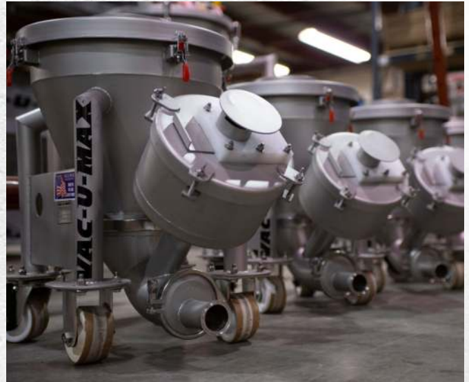
Starting with a properly designed pick-up point with phase density control impedes future issues with line plugging and inconsistent material flow.
