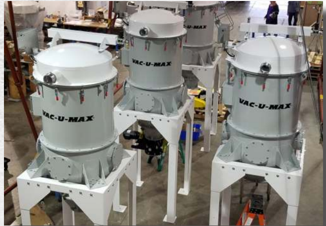
Carryover Tea Dust Captured and Safely Controlled with VAC-U-MAX Filter Separators.
