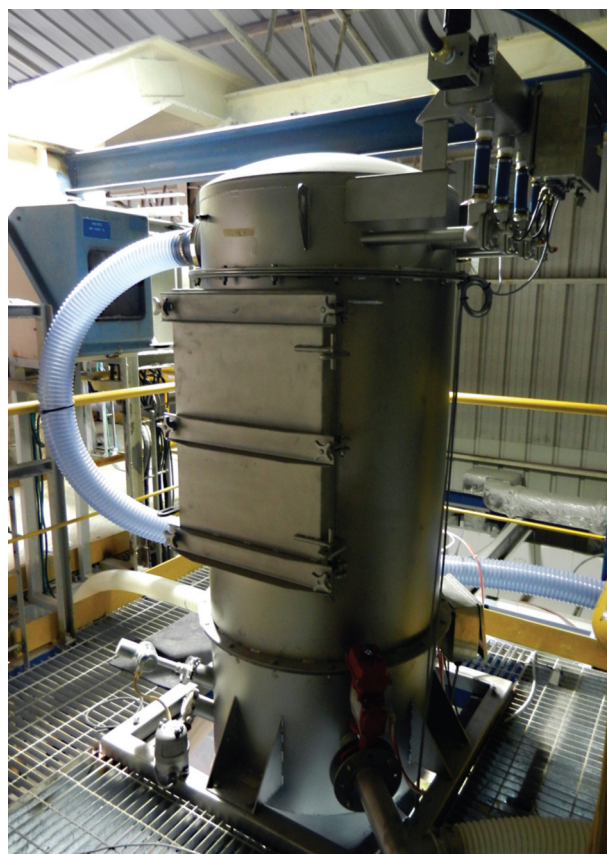
VAC-U-MAX filter receiver at Dead Sea Works LTD.
