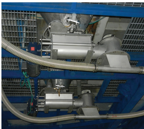
VAC-U-MAX screw dischargers metering material into vacuum conveying from large hoppers.
