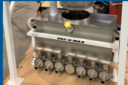
Feedbin with multiple outlets
