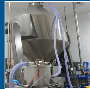
Direct Charge Loading to Mixers & Blenders
