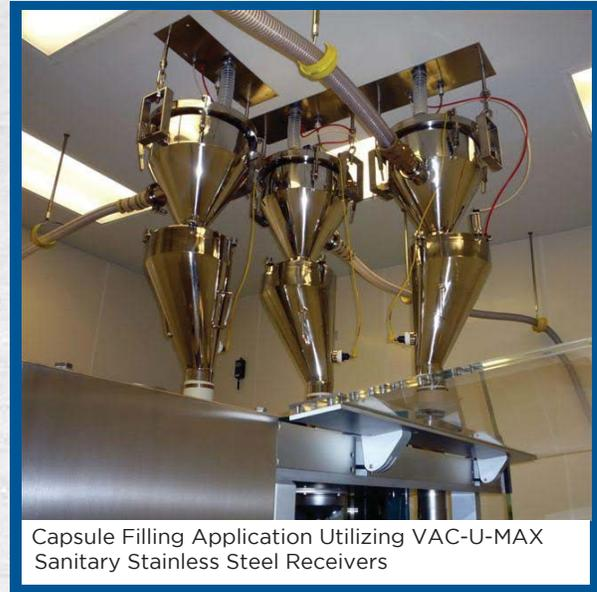
Capsule Filling Application Utilizing VAC-U-MAX Sanitary Stainless Steel Receivers
